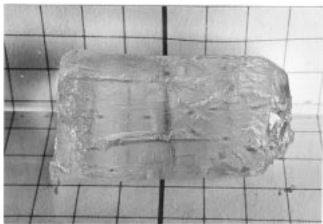
Figure 4. Microemulsion nanogel after \gamma -irradiation (62 kGy) of the system MEDDAB/styrene 10/2. The size of the sample is 3 \times 1.5 cm.
